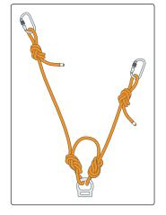
When tying this cow's tail, consider the length required to achieve the correct positioning for the work task, and the need to reach the end connector(s). It is essential that the user can reach the end connector when the cow's tail is under load.
